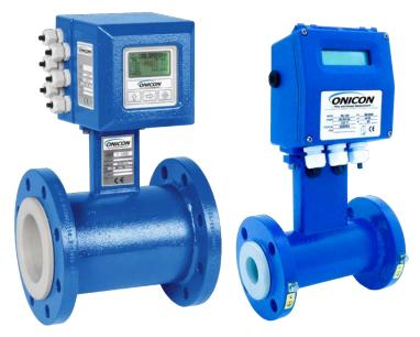
Faraday's Law states that a voltage will be induced in a conductor (the conductive fluid) when it passes through a magnetic field (generated by the meter) and that voltage will be directly proportional to the velocity of the conductor (the fluid). This voltage is measured by electrodes on opposite sides of the flow tube and used to calculate the flow velocity.
