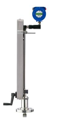
Vortex flow meters detect the frequency of alternating low pressure vortices that are formed as flow is diverted around a bluff body. These swirling low pressure zones apply lateral pressure first to one side and then to the other of sensors located downstream of the bluff body. This causes the sensors to vibrate. The frequency of this vibration is directly proportional to the flow velocity.
